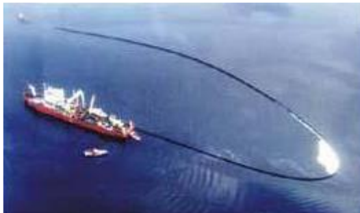
Deployment of the Vikoma weir boom
